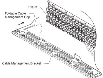
6. Fix the solid cables to the cable fixture hole using cable ties.
