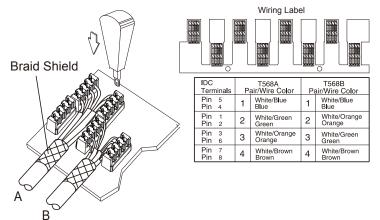
Place grounding clip on the cables, screw on the bolt until the cables are fastened to secure grounding between cable and panel. Use supplied cable ties to tight up the cables. Mount the metal cover to panel and finish the installation.
