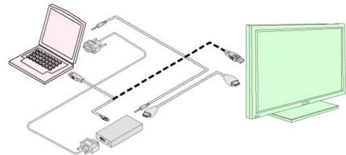
Note: If the display has an unused USB port, the VP500-101 can be powered from the USB port on the display as shown by the dashed connection.
