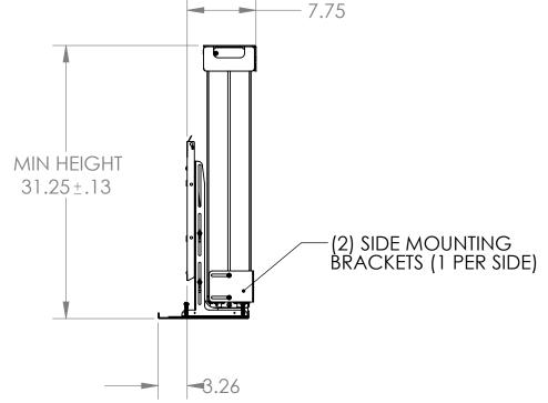
NOTE: 1. CUSTOM INTERAFCE BRACKET NOT SHOWN. THE CUSTOM INTERFACE BRACKET NEEDED FOR YOUR DISPLAY WILL ADD BETWEEN 1/2" AND 2" IN DEPTH AND MAY AFFECT LOCATION OF DISPLAY ON THE MOUNT. 2. ALLOW FOR A MINIMUM OF 1.5" OVER-HANGE ON ALL SIDES OF SHELF OVER DISPLAY.
