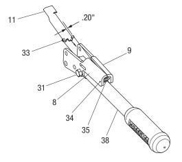
15. Insert shoulder screws (13 and 16) to align handle plates and tighten hex screws (31) to 170-190 in-lb. Remove shoulder screws.
