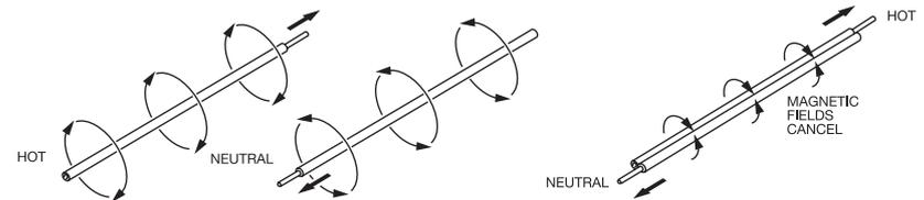
To avoid the canceling effect of the opposing magnetic fields and optimize the transmitted signal, the conductor to be traced should be separated from the return conductor by utilizing a remote return path.
