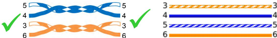
If the error is repaired at the wrong end of the cable, the end-to-end continuity is corrected, but a split pair is formed:
