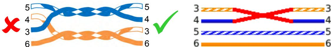
If the error is repaired at end of the cable where the fault is located, the fault is removed:
