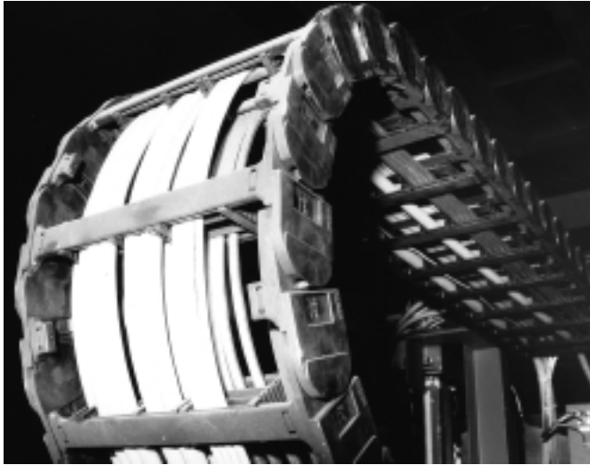
Flat cables and pneumatic hoses installed in an Energy Chain® with full interior separation of all cables.
