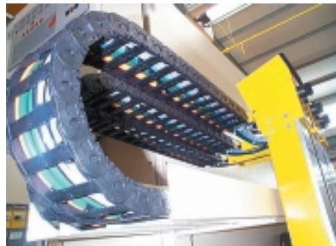
igus Chainflex® cables permit the smallest bending radius of 5 \times d for one million strokes
