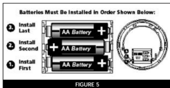
**CAUTION!** Alarm will not engage to bracket unless all three batteries are installed. Removal of any or all batteries will render the alarm inoperative!
