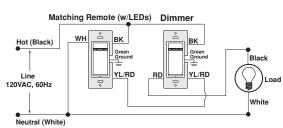
NOTE: The dimmer must be installed in a wall box that has a Load connection. The matching remote must be installed in a wall box with a Line Hot connection and a Neutral connection. A Neutral wire to the matching remote needs to be added as shown If you are unsure about any part of these instructions, consult a
