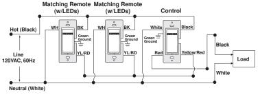
NOTE: The control must be installed in a wall box that has a Load connection. The matching remote must be installed in a wall box with a Line Hot connection and a Neutral connection. A Neutral wire to the matching remote needs to be added as shown.
