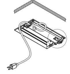
Loop cord to nearest cord clip Note: In a conduit application; conduit should be supported according to local code.
