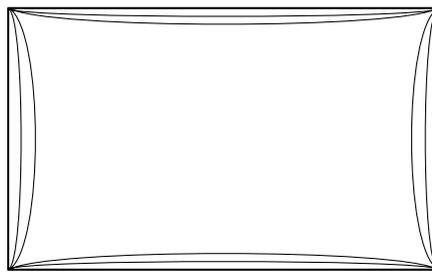
**Square or Rectangular Ducts:** The expanding metal wants to expand longitudinally but cannot, thus it deflects inward, creating an opening around the duct
