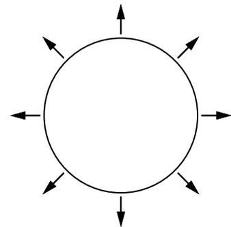
**Round Duct:** Stronger due to its geometry, the duct cannot collapse inward and thus tends to expand.
