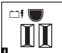
4 Battery Backup/Surge Protected Outlets
